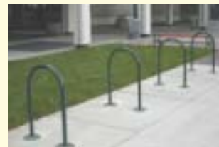
The inverted-U bike rack, whether as stand-alone units or on rails with multiple Us, make for excellent bike parking when the inverted Us are spaced at least 30 inches apart. Two bikes can use each inverted U.
